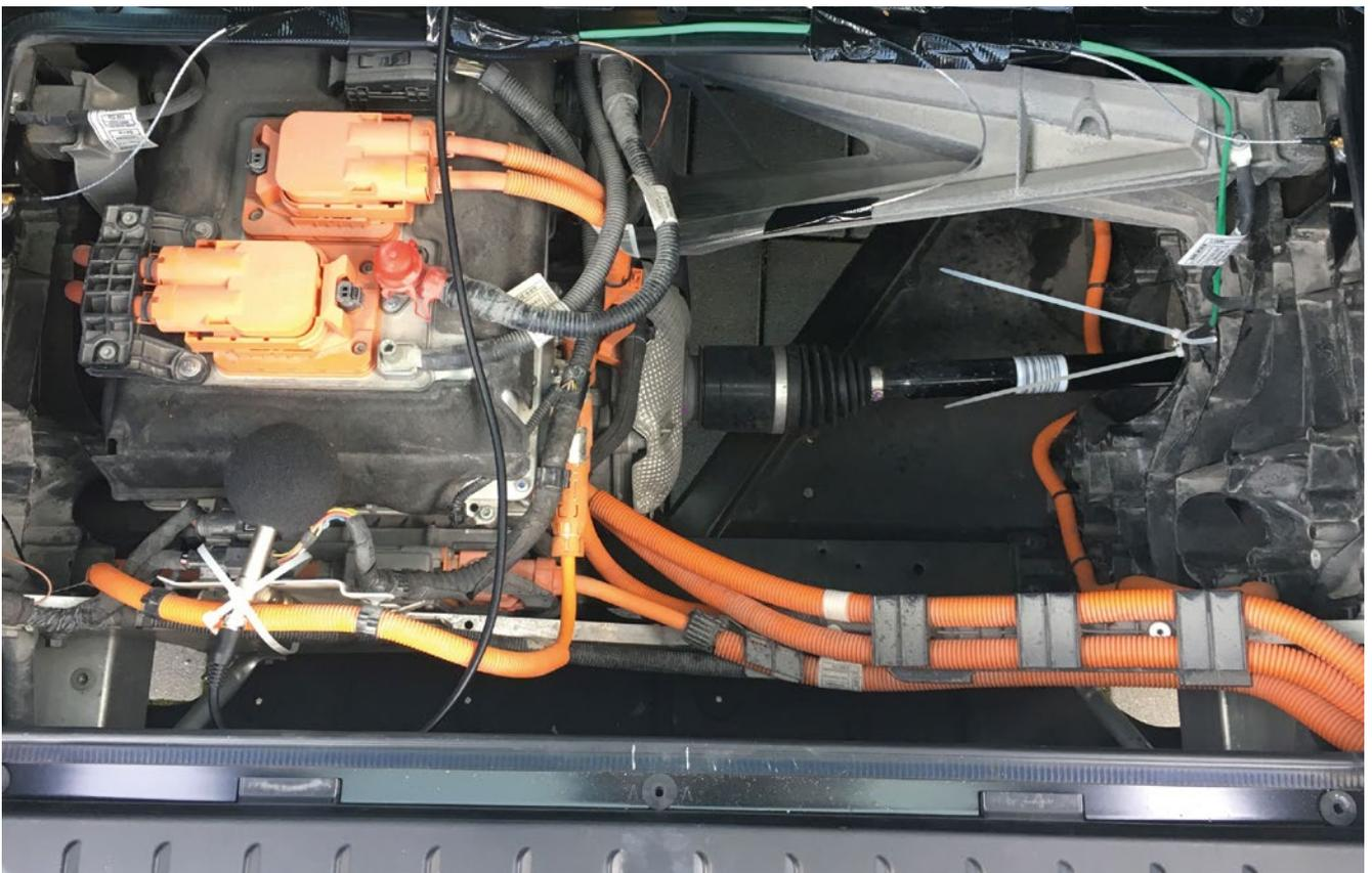
**FIGURE 1** Both engine and gear box are combined as a drive unit, with almost no chance to acquire rotational speed (© Müller-BBM)
