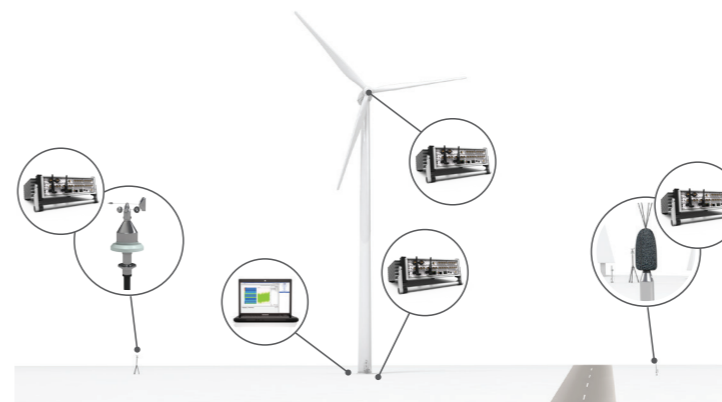
Figure 12: An exemplary wireless distributed data acquisition system for wind turbines
