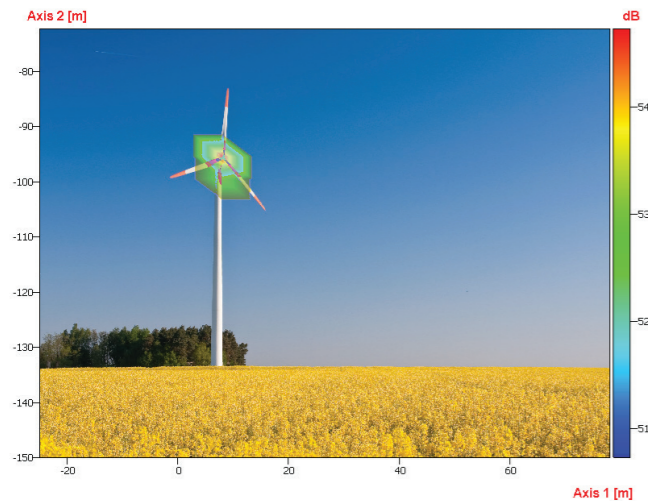
Figure 6: A localized sound emitted by the generator of a wind turbine
