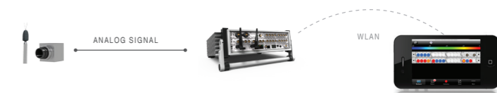
Figure 13: Exemplary setup of PAK capture suite with an iPhone as monitoring and configuration device
